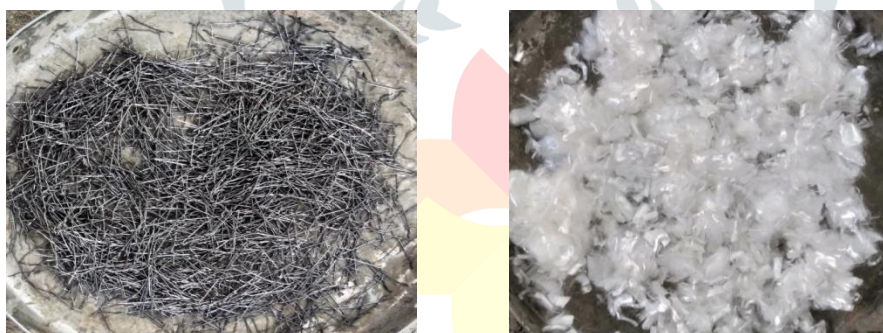
Fig.1 Steel fibre and Polypropylene fibre.
