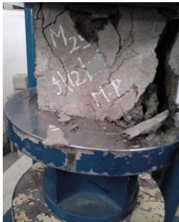
Fig 6.2 Concrete cube specimen in after testing
