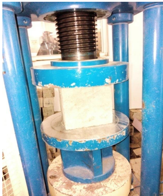
Fig. 6.1 Compressive Strength Testing for Cube
