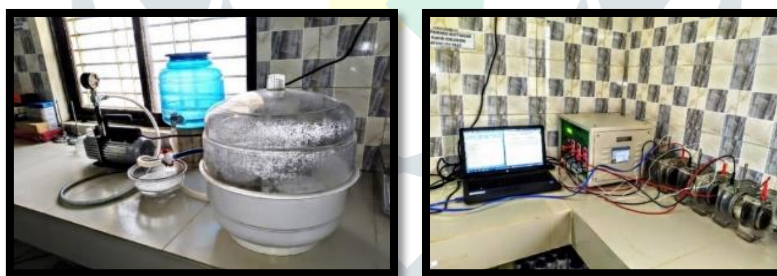
Figure-2: RCPT test of concrete as per ASTM C1202
