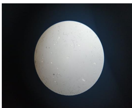
Figure 3. – Formation of Crystals without inhibitor
