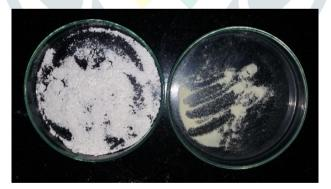
Figure 1 Bulk ZnO (Left) and synthesized ZnO nanoparticles (Right)
