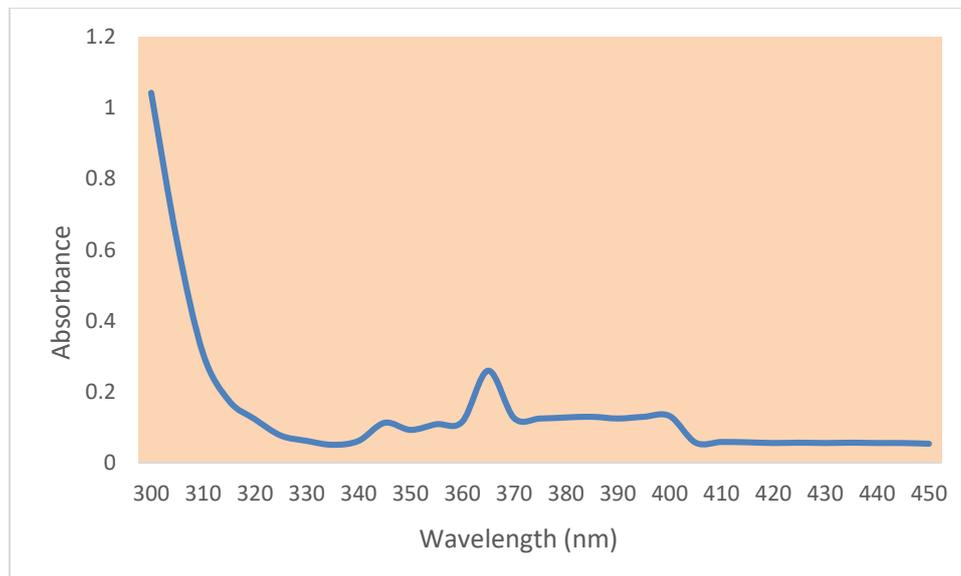
Figure 2 UV-Vis spectrum of ZnO NPs
