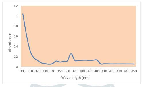
Figure 2 UV-Vis spectrum of ZnO NPs
