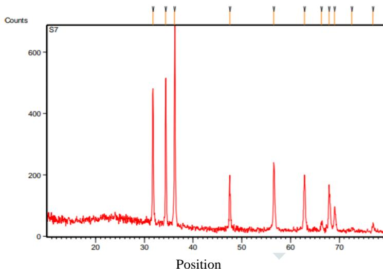
Figure3 XRD Spectrum of ZnO NPs
