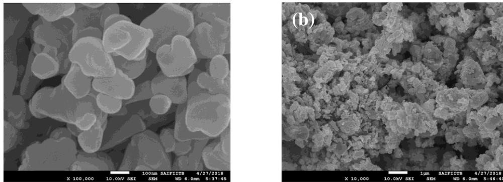
Figure 4 SEM Images of ZnO NPs in different magnification ranges (a) 100nm (b) 1µm.
