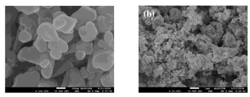
Figure 4 SEM Images of ZnO NPs in different magnification ranges (a) 100nm (b) 1µm.
