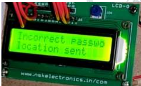
Figure 9: If incorrect OTP is entered system sends the vehicle location
