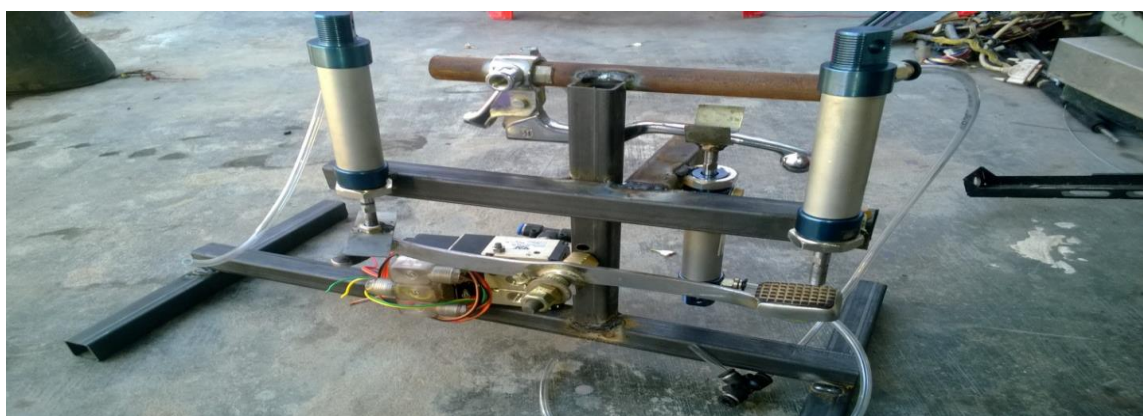
Fig 13: Experimental Model of Automatic Gear Changer
