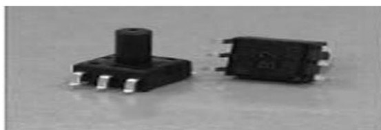
Fig 3.3 Blood pressure sensor MPS-3117
