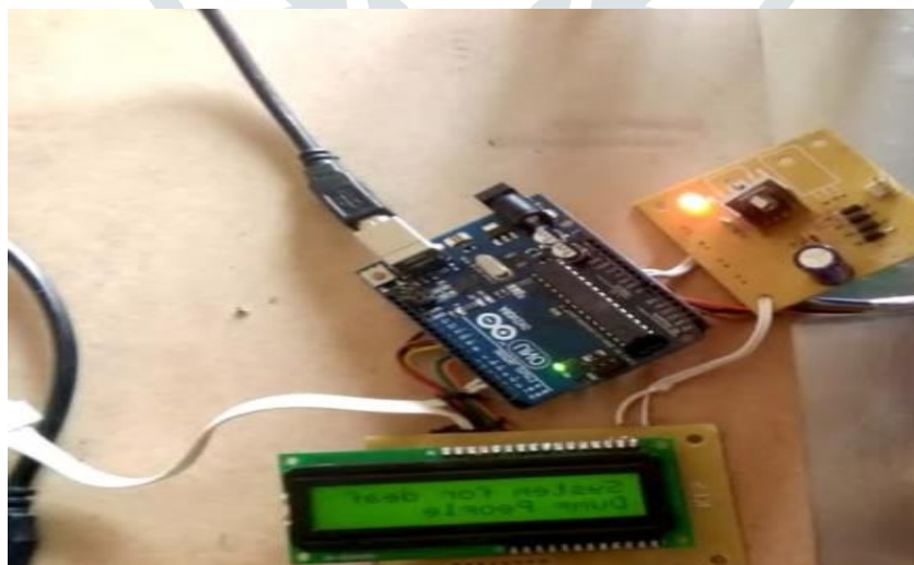
Fig 2.5 : System working with Flex Sensor
