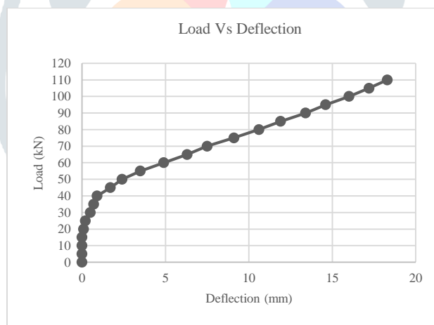
Fig. 8 Load Vs Deflection curve for Specimen 1 from 3 rd phase
