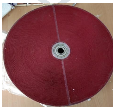
Fig. 6 Desiccant Wheel having Sinusoidal Geometry(1:1)
