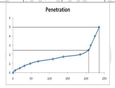
Load at 2.5mm penetration = 207kg, Load at 5mm penetration = 235.75kg CBR value at 2.5mm penetration = (penetration load/ standard load)\*100 = (207/1370)\*100 = 15.11%
