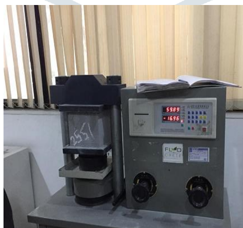
Fig 2: Compressive Strength Test.
