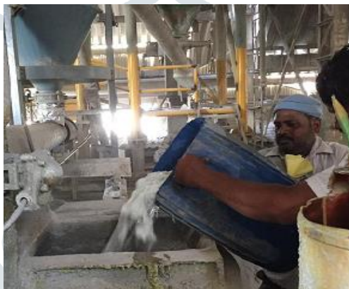
Fig 1: Pouring of plastic waste in the mixture
