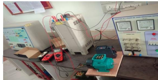
Fig.4: Prototype model three phase induction motor without VFD
