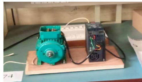
Fig 2: Prototype model three phase induction motor with VFD
