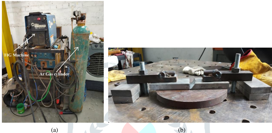
Figure 2: (a) Experimental Setup for TIG welding, (b) Fixture of the work piece
