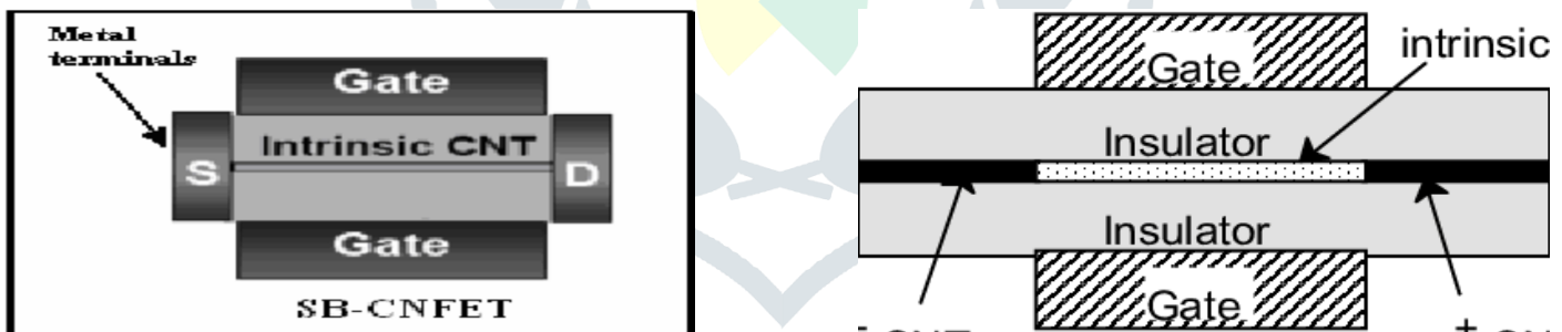
Fig. 1. Different types of CNTFETs: (a) Schottky barrier (SB) CNTFET (b) MOSFET-like CNTFET.[7]
