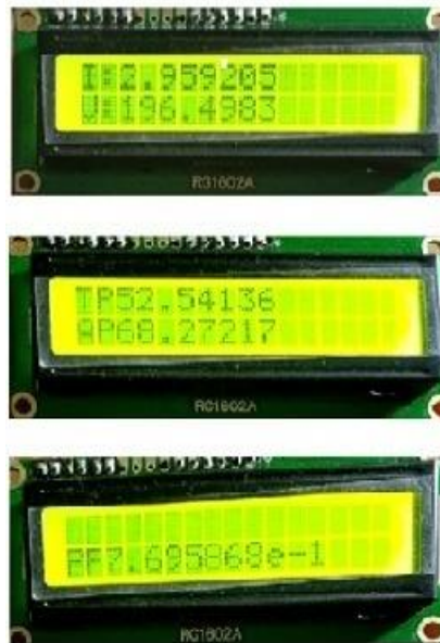
Figure 7. Load condition after power factor correction
