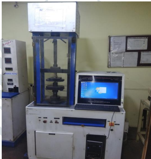
Fig.1 computerized spring endurance testing machine
