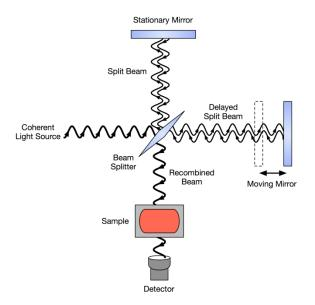
Fig.2: Schematic diagram of a Michelson interferometer, configured for FTIR
