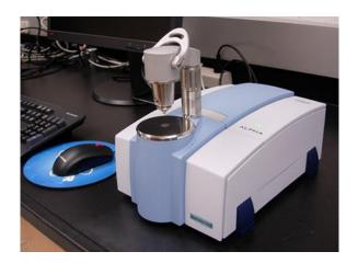
Fig.3: FTIR Spectrometer
