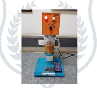
Fig.1: Mechanical stirrer used for blending base oils with synthetic oil
