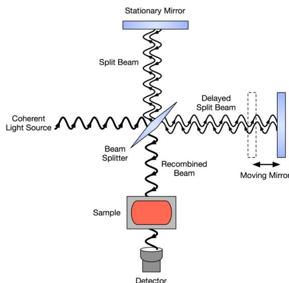
Fig.2: Schematic diagram of a Michelson interferometer, configured for FTIR
