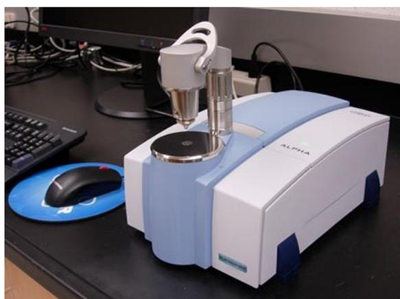
Fig.3: FTIR Spectrometer
