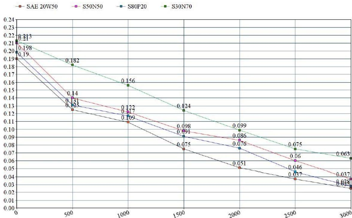
Fig.8: Variation of the coefficient of friction with a sliding distance
