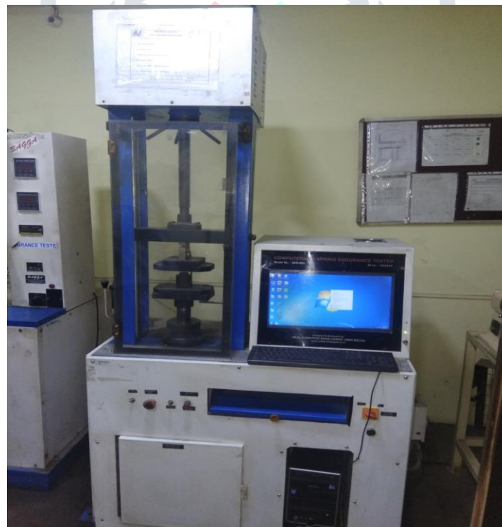
Fig.1 computerized spring endurance testing machine
