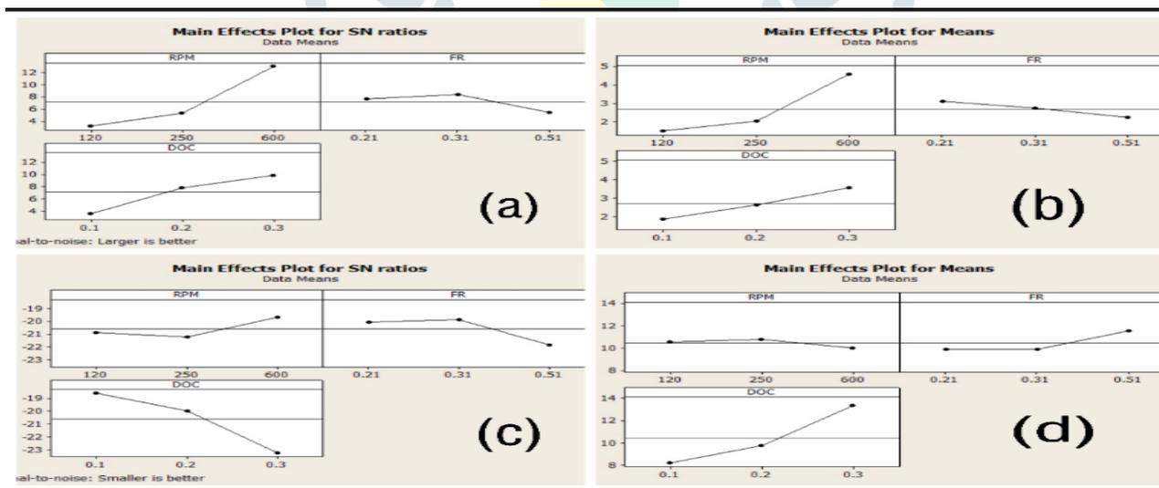
Fig.1: Main effect plot for the cutting force and material removal rate (MRR) uncoated carbide tool (a) S/N ratio of MRR (b) mean of MRR (c) S/N ratio of cutting forces (d) mean of cutting forces
