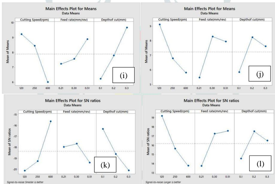
Fig.3: Main effect plot for the cutting force and material removal rate (MRR) TiAlN coated tool (i)Means of CF, (f)mean of MRR (k) S/N ratio of CF (l) SN ratio of MRR
