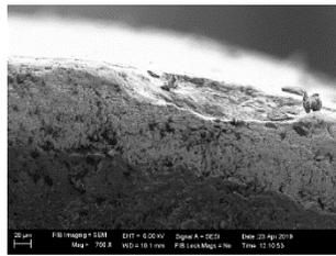
Fig.5:TiAlN coated tool under sem analysis at 750x
