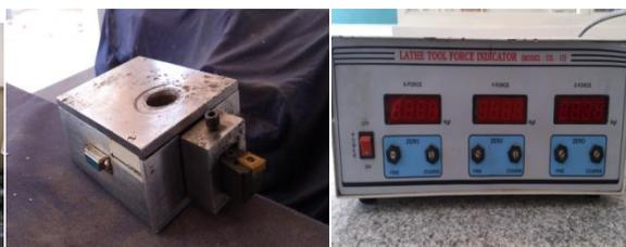
Fig.3: Lathe Tool Dynamometer
