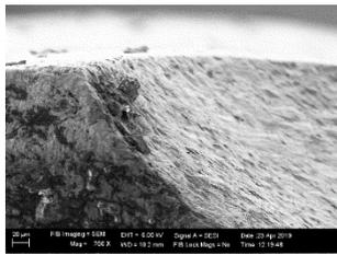
Fig.4:Uncoated tool under sem analysis at
