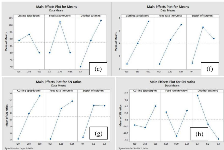
Fig.2: Main effect plot for the cutting force and material removal rate (MRR) AICrN coated tool (e) Means of CF, (f) mean of MRR (g) S/N ratio of cutting forces (h) SN ratio of MRR
