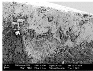
Fig.6:AlCrN coated tool under sem analysis at 750x
