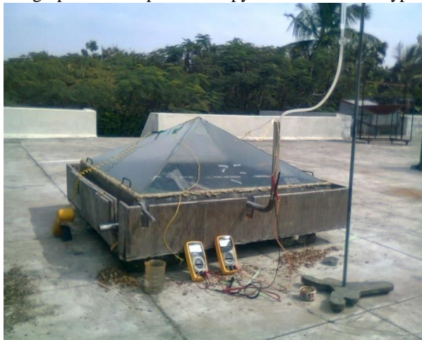
Fig. 2 Photograph of the experimental pyramid tilted-wick type solar still
