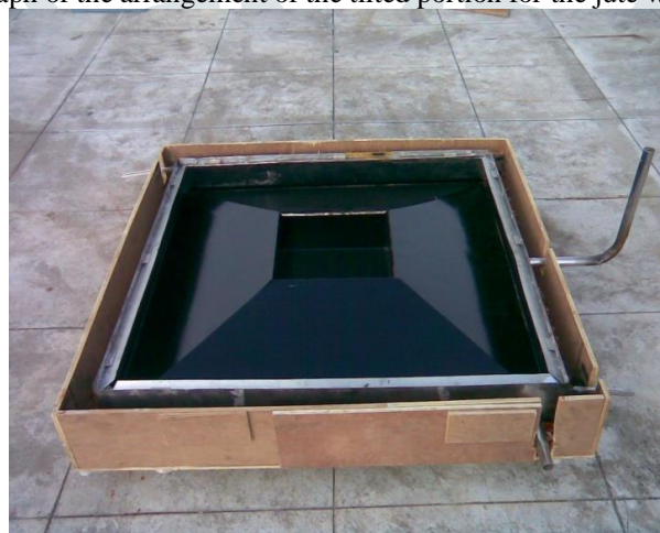
Fig. 1 Photograph of the arrangement of the tilted portion for the jute wick to be spread
