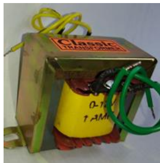
Fig No.2 Transformer
