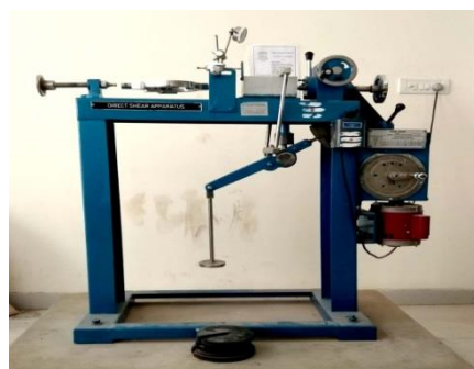
Figure 2 Direct Shear Box
