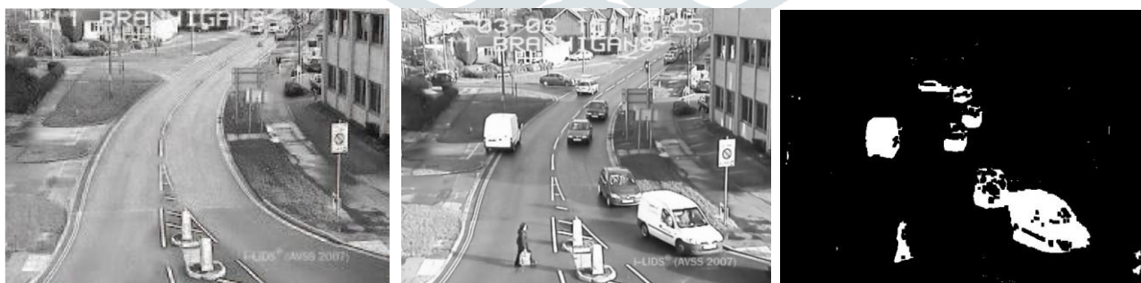
Fig 2: An example of parked vehicle where the first image is the reference background model, Second image is the current background model and the third image is the dual background model subtraction result
