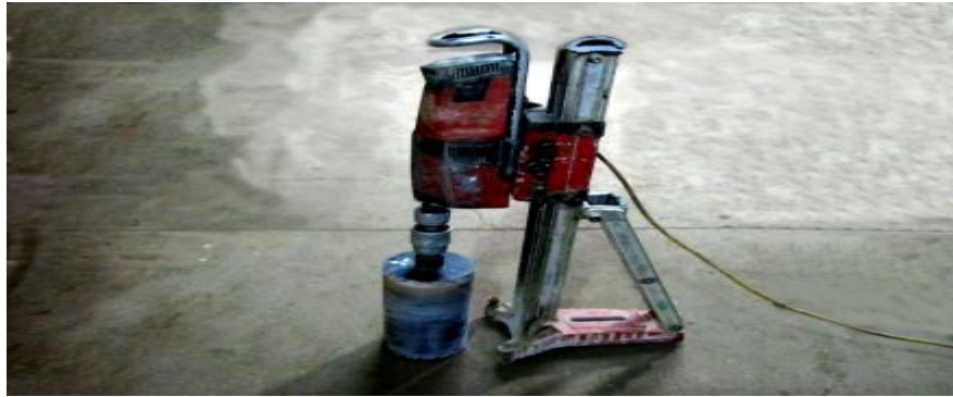
Core drilling machine
