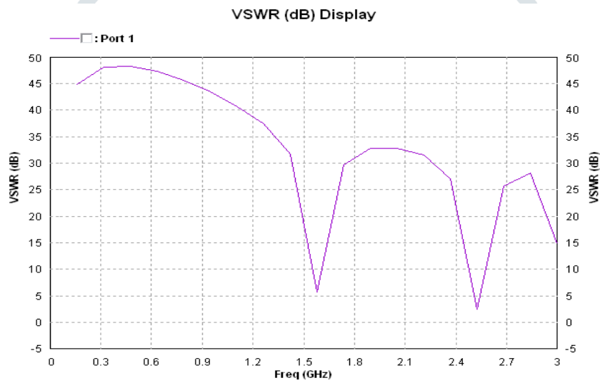
Fig. 3: VSWR Graph v/s Frequency
