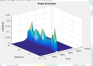
Step 3: Pulse broadening Ratio: It is spreading of the light pulses as they travel down the fiber.
