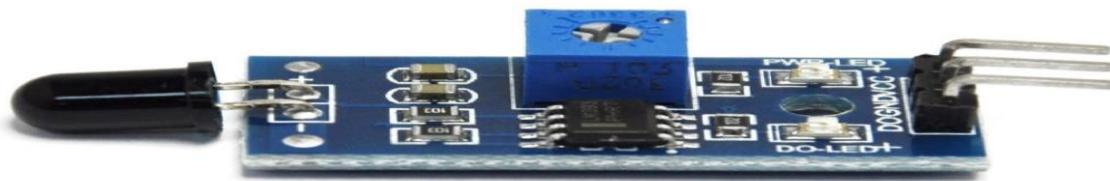
Fig no 11: Flame Sensor infrared Receiver Ignition source detection module
