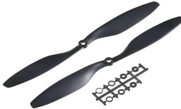
Fig5: Reinforced carbon fiber based propellers
