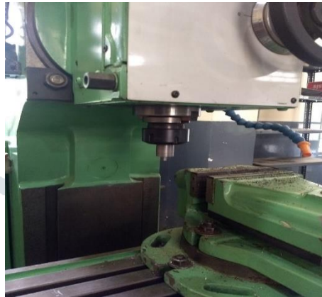
Figure 1: Tool Setup in Vertical Milling Machine
