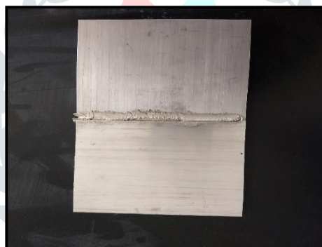
Figure 2: Aluminium Welded Joint without Silicon Carbide
