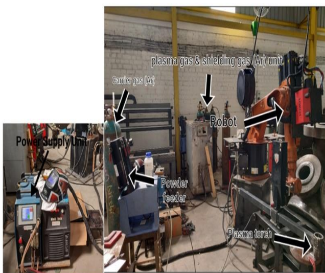
Figure 1 Automating robotized plasma arc welding setup
