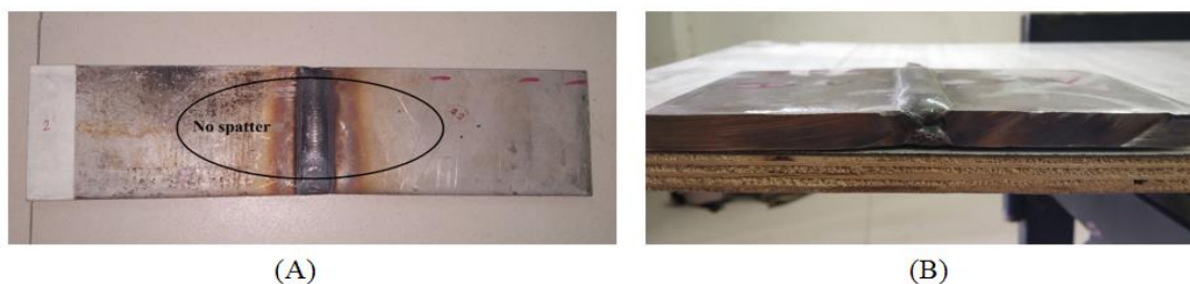
Figure 2 (A) Free from spatter, (B) Free from distortion
