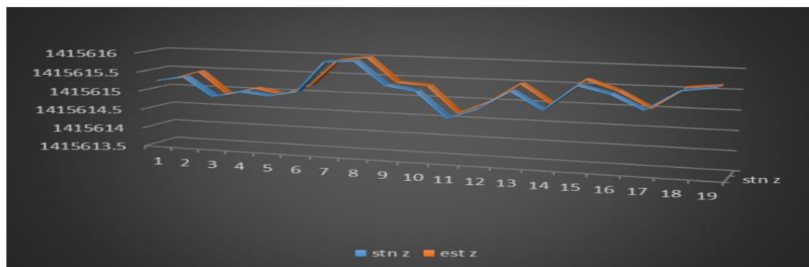
Figure 9: comparison of estimated receiver position and receiver position observed from the NavIC receiver As seen from the above graph the estimated and observed receiver position are almost equal when satellite clock correction is considered.
