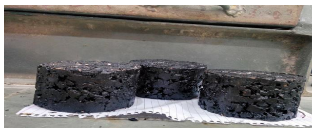
Figure 2 Marshall Sample of SMA Mixture
