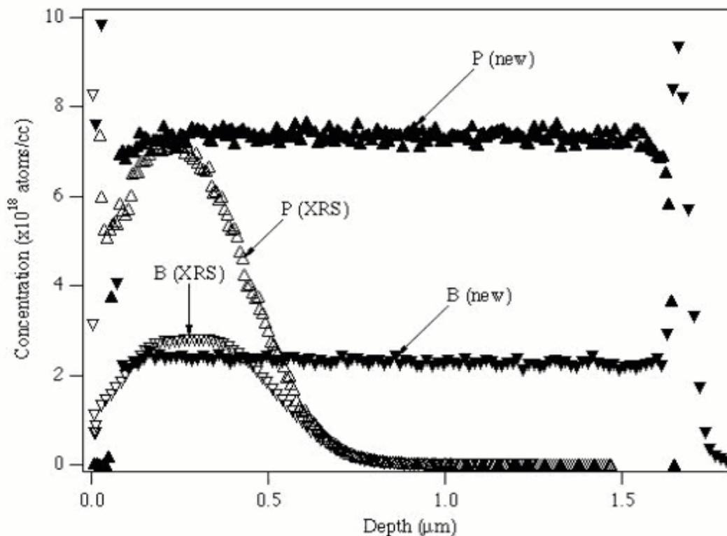
**Figure 2.** SIMS measurement of a traditional Si implant (empty triangles) and of a diffused Si implant (full triangles). The peaks at the two sides of the implant are just an artifact of the SIMS measurement.
