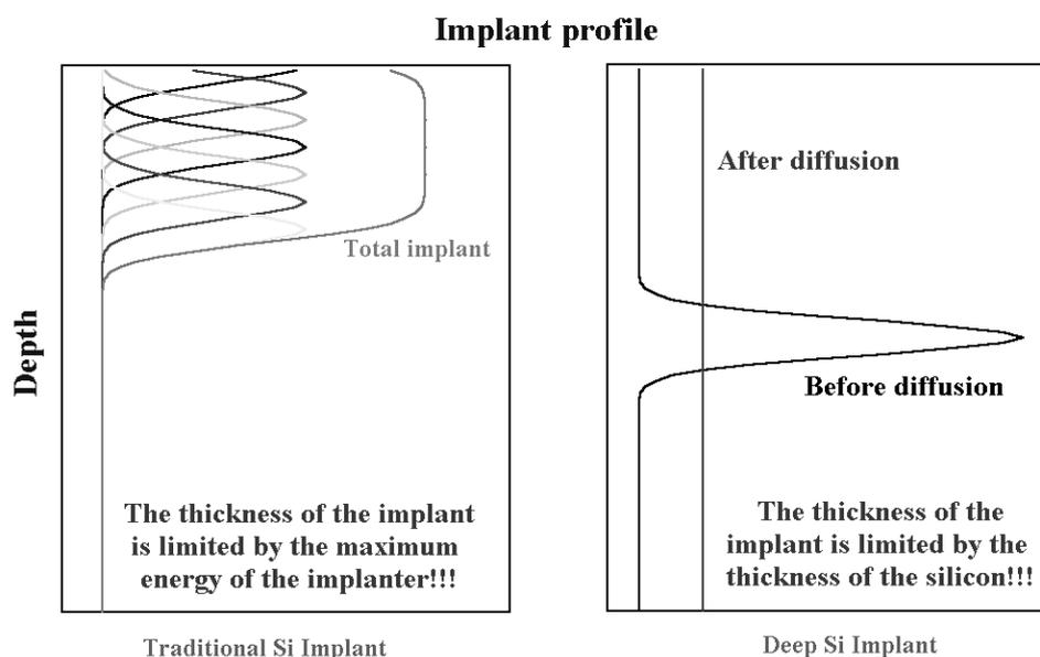
**Figure 1.** Schematic view of implant profile in traditional Si implant (left) and in diffused Si implant (right).
