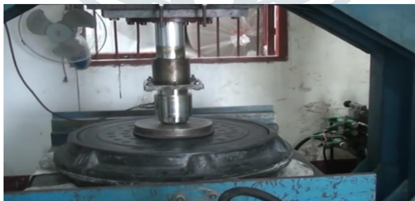
Figure 5. Test setup for testing of manhole cover in UTM
