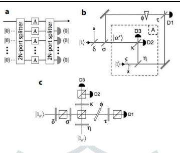
So as to check that amplification has happened, we utilized photon tallying to think about the deliberate normal photon number at the info what's more, yield of the amplifier stage the deliberate force gain, g 2, as an element of the increase control reflectivity  $\eta$ , contrasted and the hypothetical qualities, when  $|\alpha 0| 2 = 0.02$ .
