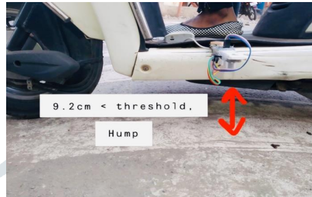
Figure 4.2. Detection of Hump
