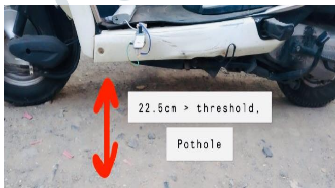
Figure 4.3. Detection of Pothole
