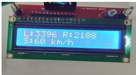
Fig.6 The LCD screen on the transmitter module displaying the distance between itself and the subsequent cars
