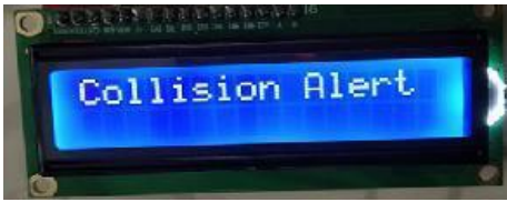
Fig.8 Collision alert on transmitter and receiver when the distance gets less than the threshold value
