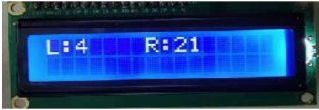
Fig.9 Distance shown after collision alert message shows that vehicle on left is near to the front more than the allowed safe limit
