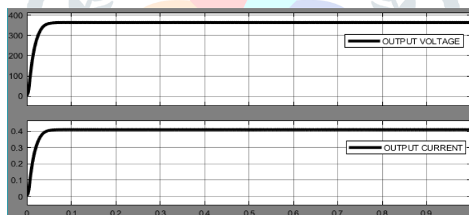
Fig 10: Output voltage and output current waveform of the proposed IBC with Closed loop system
