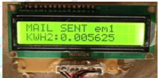
Fig. 9 LCD display showing Energy Meter 2 Readings
