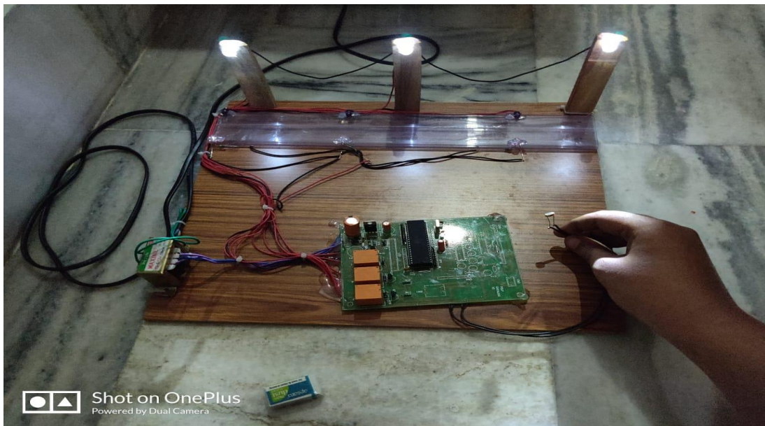
Fig 4: With 50 percent intensity (Low light intensity falling on LDR)
