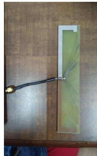
Figure 3: Fabricated micro strip antenna
