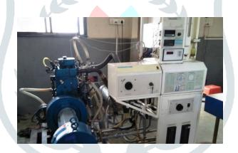
Make- Kirloskar, Power-3.50Kw, Speed-1500 rpm, No. of Cylinder-1 (Single Cylinder), No. of Stroke-4-Stroke, Type of Cooling-Water Cooled, Fuel-Diesel, Cylinder Bore-87.50mm, Stroke Length-110mm, Connecting Rod Length-234mm, Compression Ratio-18.00, Swept Volume-661.45cc.
