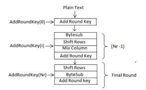
It performs substitute, Shift rows and Mix columns and Add Round Key operations in each round except the last round where Mix column operation is skipped[4]. AES can be easily implemented in software as well in hardware for cryptography.
