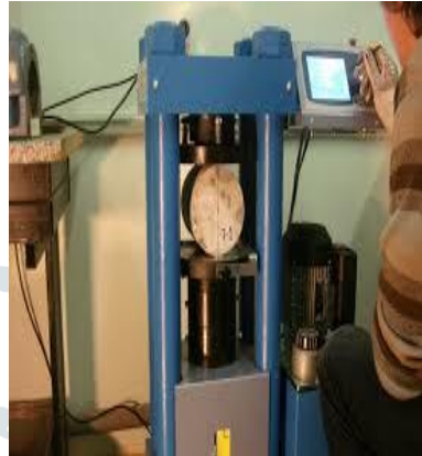
Figure : Split tensile test
