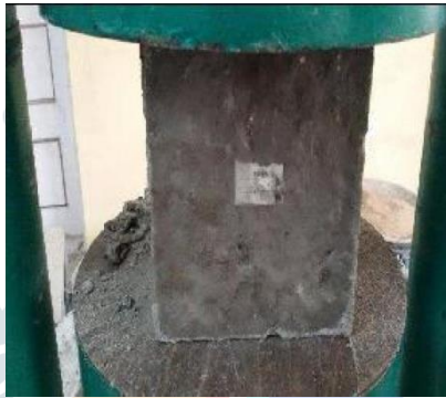
Figure : Compressive strength on cube
