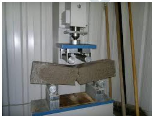
Figure : Flexural Strength test on Beams
