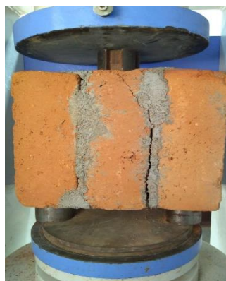
Fig 2.3 Experimental set up for Shear Testing
