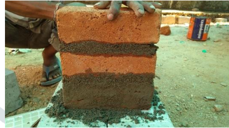
Fig 2.1 Preparation of a brick triplet
