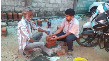
Fig 2.1 Preparation of a brick triplet
