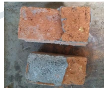
Fig 3.3 Partial bond and partial brick failure.
