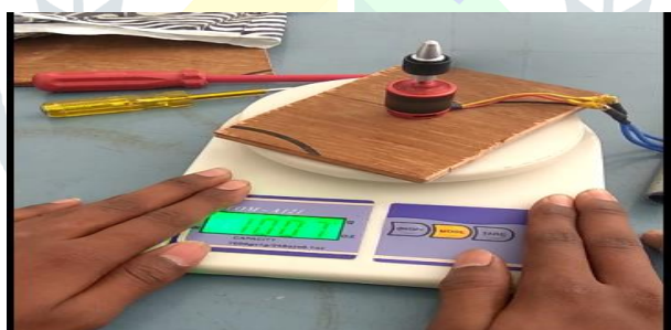
Fig.6 Thrust measurement set-up
