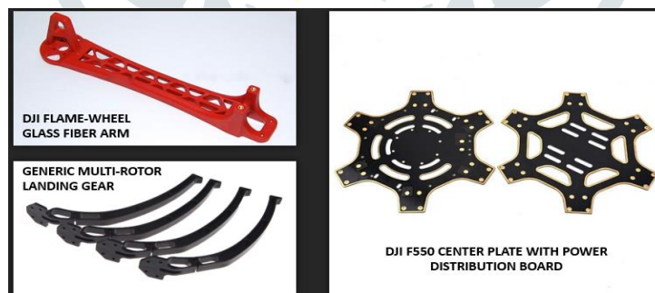
Fig.10 components of frame
