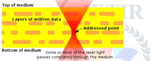
Figure a): A schematic diagram showing a cross-section of an optical 3D storage
