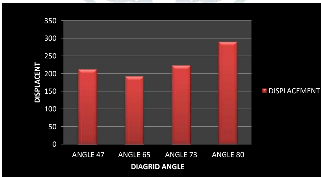
Figure 12: Displacement of Hexagonal Building at various angles
